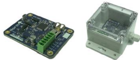
Figure 6: Seaview Wave Sensor SVS-603
